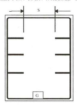
GATE 21 X 25 MILS: SOURCE CONNECTION CENTRALLY BETWEEN INDICATOR LINES: 89 MILS
